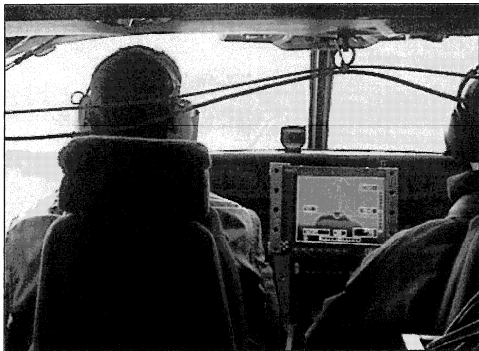
Figure 6-6 Position of wake display between pilots.
