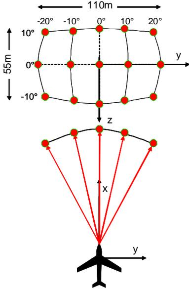
**Figure 7. Forward looking sensor onboard implementation with 15 measurement directions**
