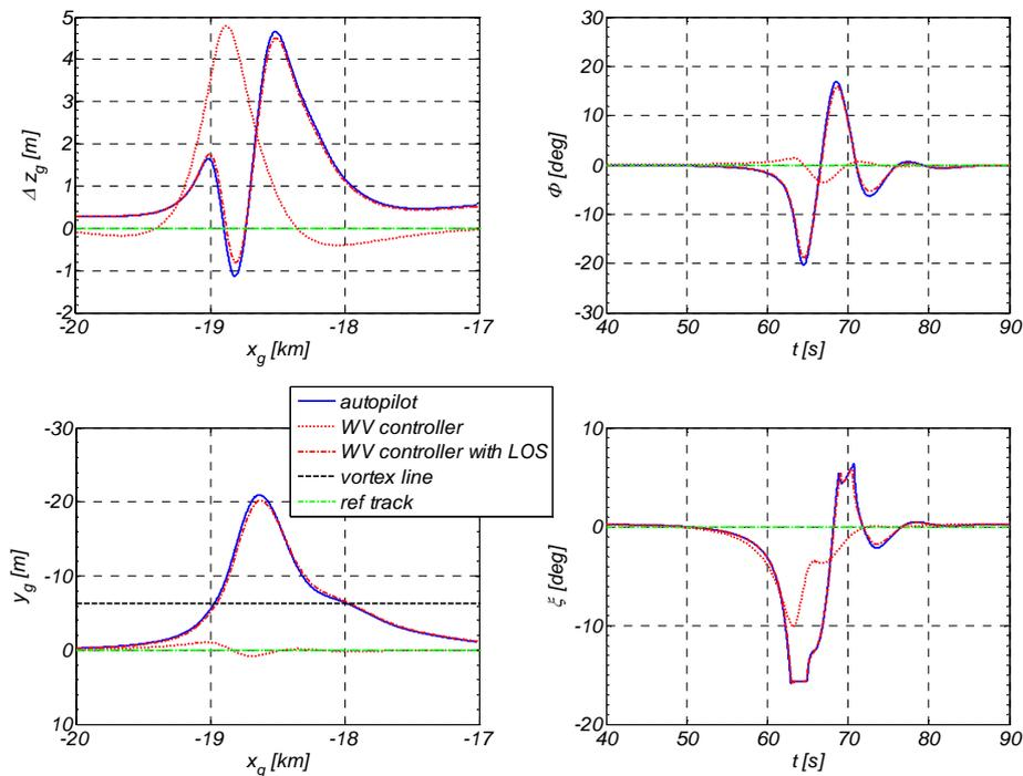
**Figure 6. Flight track and time histories of a flight through wake vortex flow field (offline simulation with autopilot exclusively and autopilot supported by wake vortex controller and with and without line of sight effect of LIDAR)**
