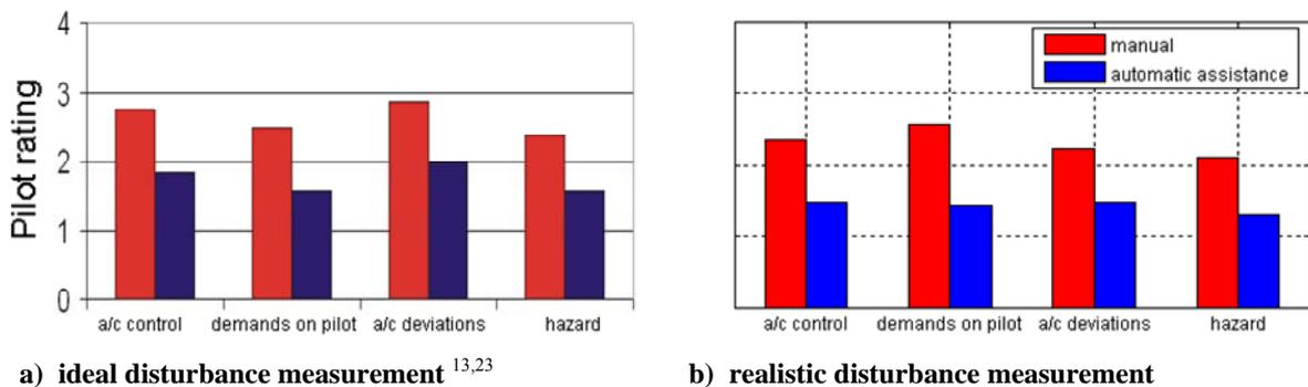
**Figure 13. Average pilot ratings for IFS wake vortex encounters**
