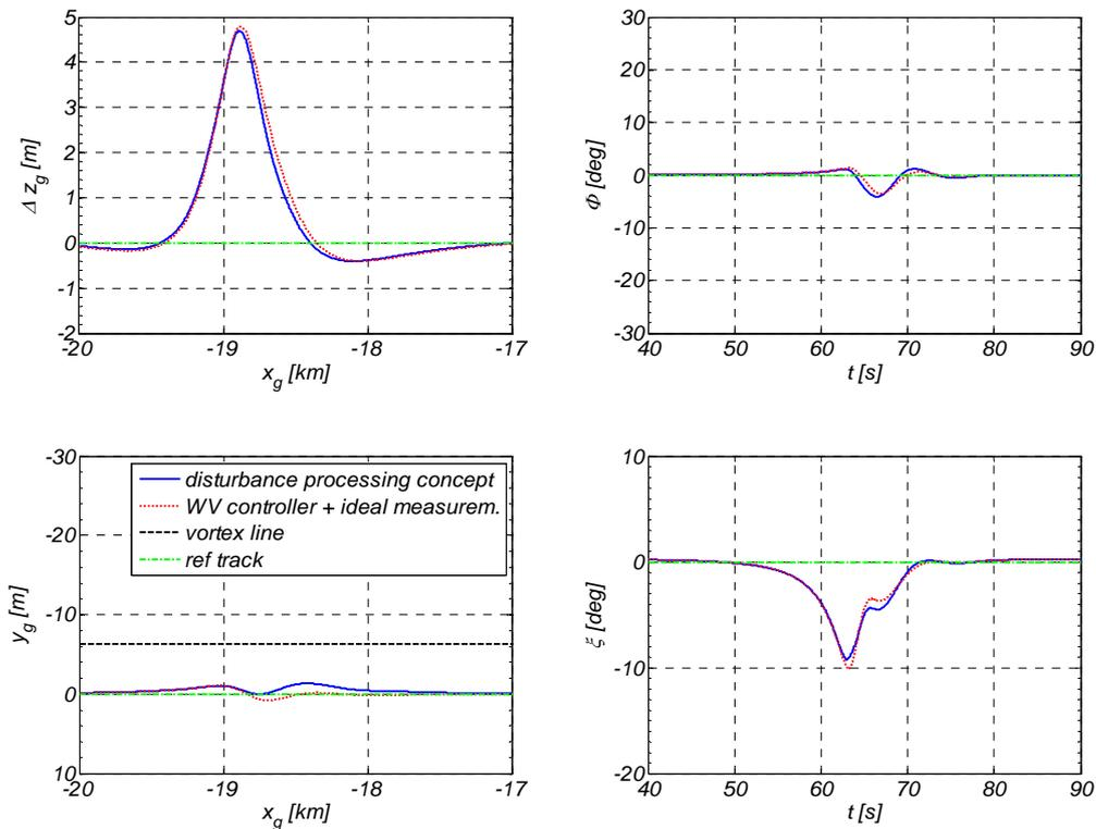
**Figure 10. Flight track and time histories of a flight through wake vortex flow field (offline simulation with autopilot supported by wake vortex controller and with and without line of sight effect of LIDAR)**
