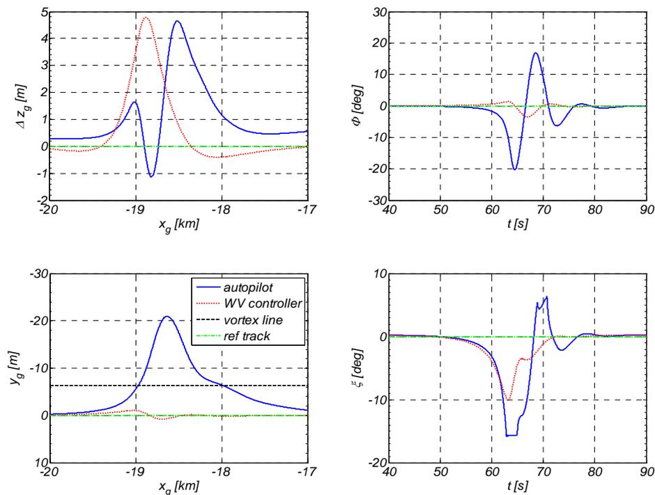
**Figure 4. Flight track and time histories of a flight through wake vortex flow field (offline simulation with autopilot exclusively and autopilot supported by wake vortex controller)**
