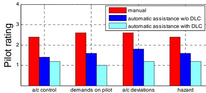
**Figure 14. Average pilot ratings for IFS wake vortex encounters with IRLIS**
