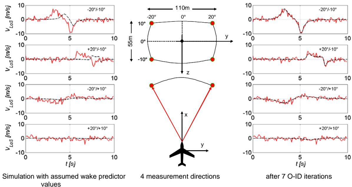
Figure 9. LoS “measurements” (—) compared to reconstructed LoS time histories (-----)
