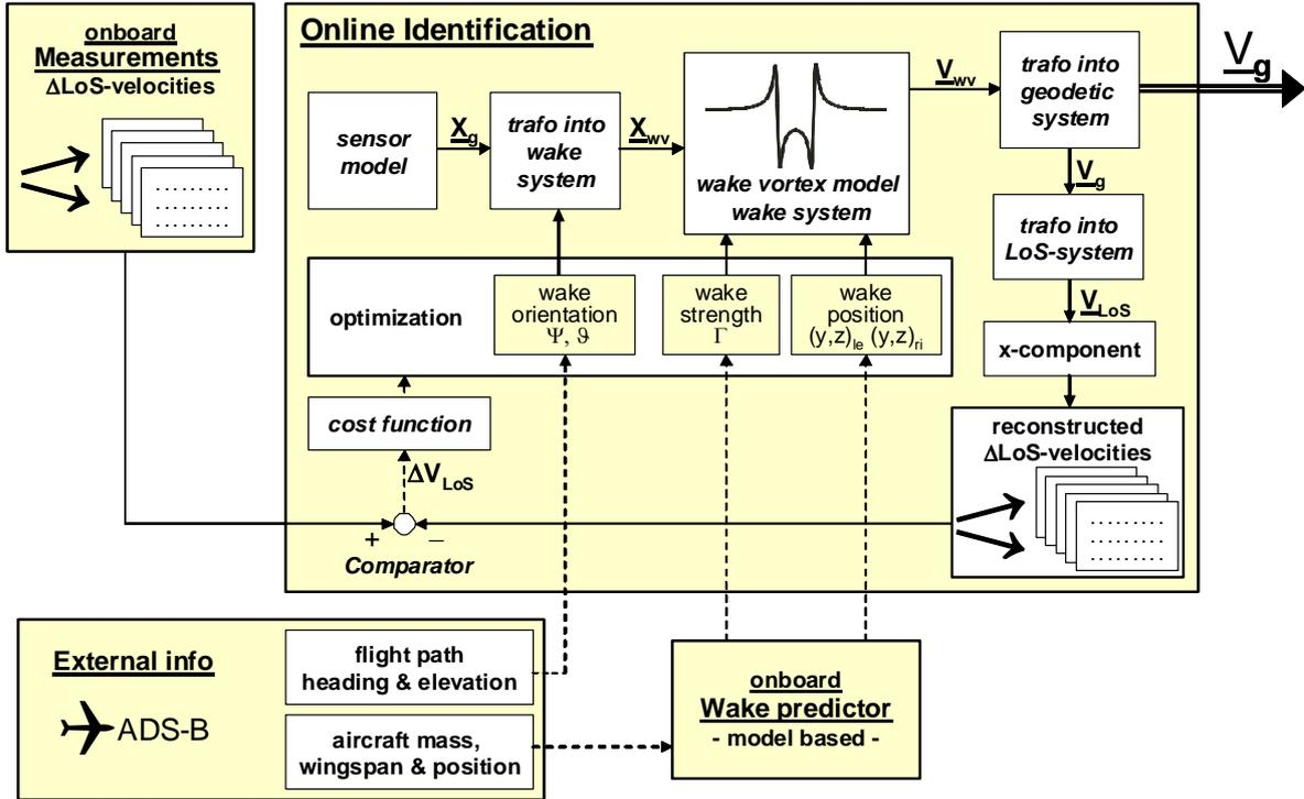
Figure 8. Concept for determination of wake vortex strength, position and orientation from Line of Sight measurements (patent pending)
