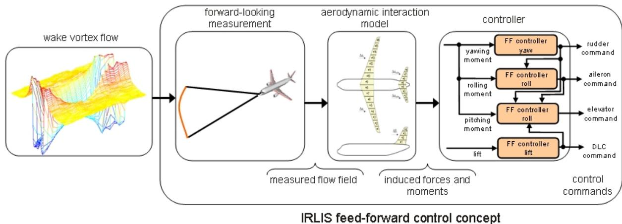
**Figure 2. Principle of the IRLIS flight control assistance system**
