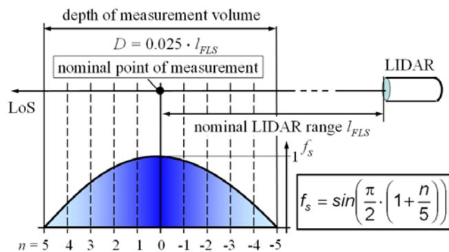
**Figure 3. Sinusoidal shaping function for measurement points of a LIDAR measurement volume along the LoS in the vicinity of the nominal LIDAR range**
