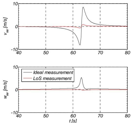
**Figure 5. Ideal disturbance knowledge compared to in Line of Sight (LoS) measurement**
