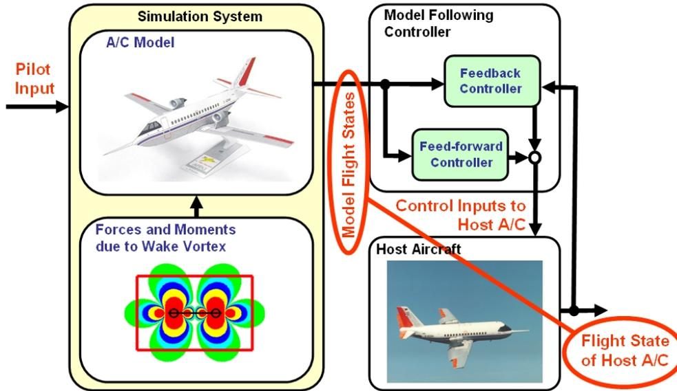
Figure 11. In-flight simulation concept
