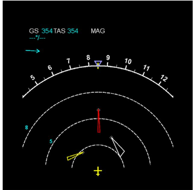
Figure 3 Wake Vortex Visualization in the ND
