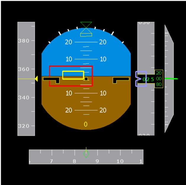
Figure 2 Wake Vortex Visualization in the PFD
